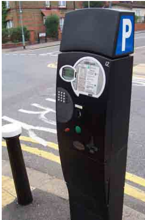
Solar Powered Pay and Display Parking Meter.
