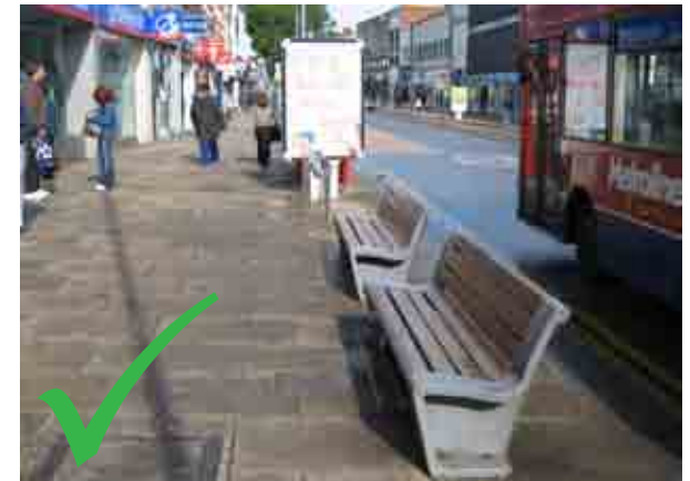
Good practice – furniture located on the kerb side, maximising clear width for pedestrians (Wood Green Town Centre).
