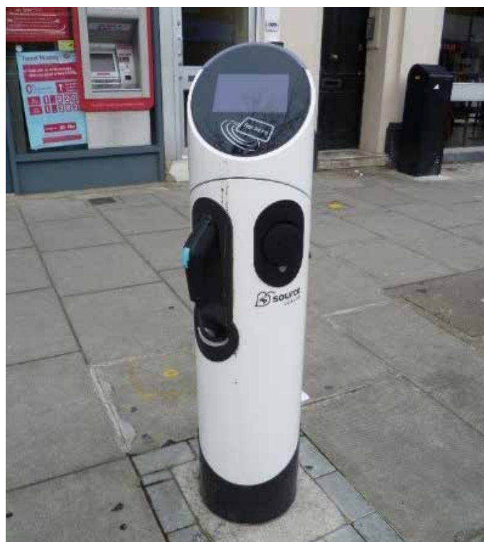
Figure 2. Fast 7 kW charging unit. (Source: Source London)
