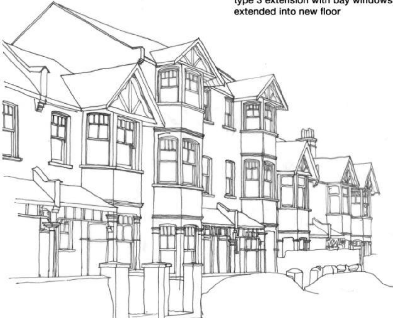
Figure 8 above:- Example of a Type 3 extension to 2 houses with the bays of both extended.
