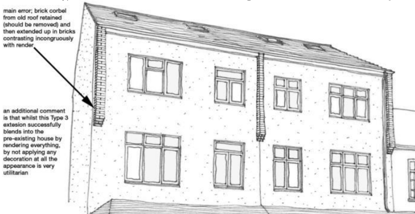
Figure 12 above:- existing party wall parapet not removed All new extensions with a parapet should match the existing next door parapets in materials and detailing.
