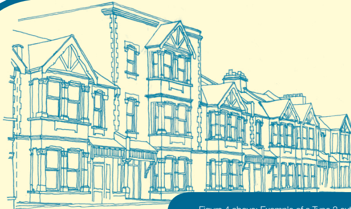
Figure 4 above: Example of a Type 2 extension with the bay extended up to the parapet.
