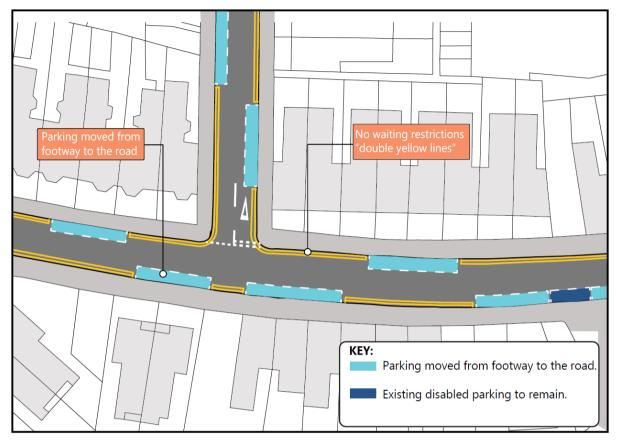
This option is proposed because pavements are less than 2 metres wide, and the road is not wide to move all parking onto both sides of the road. Parking on the road is proposed on both sides for limited lengths and staggered along the road.
