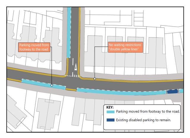
This option is proposed because pavements are less than 2 metres wide, and the road is not wide to move all parking onto both sides of the road. Parking is proposed on the side of the road that best meets demand and is safe.
