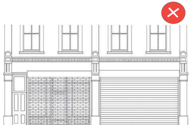
Picture 68. External Roller shutters are not appropriate.
