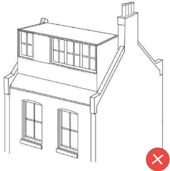
Picture 71. Over-sized dormers will not usually be acceptable in the conservation area.
