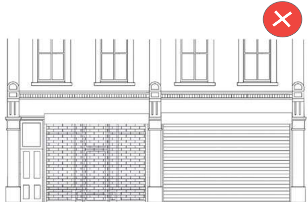
Picture 66. External Roller shutters are not appropriate.
