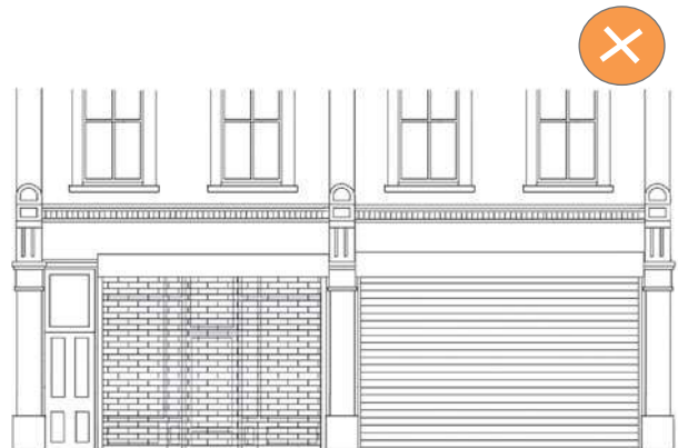
Picture 48. External Roller shutters are not appropriate.
